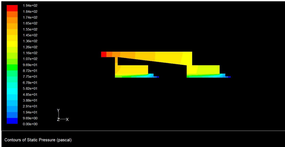
Figure 18: Fluent improved channel design results
