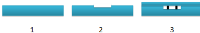
Figure 11: Laser cut PMMA fabrication process
