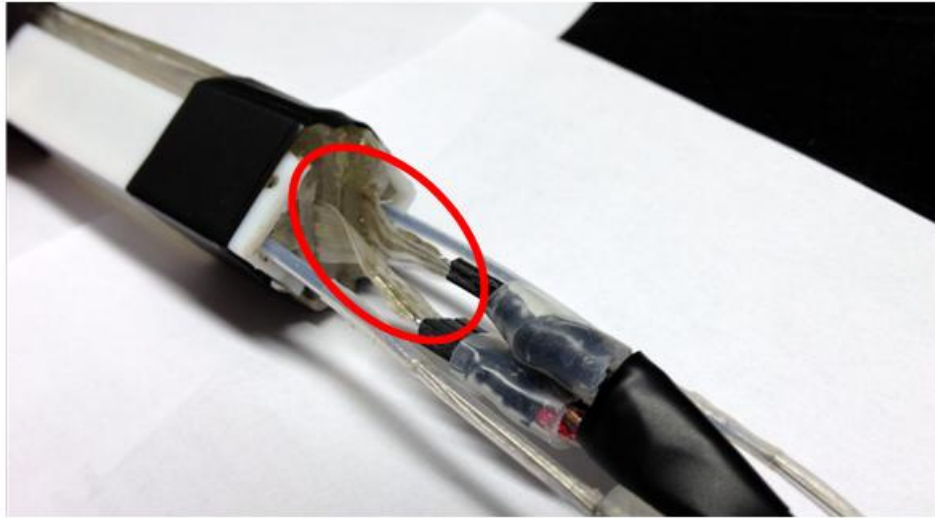
Figure 23: Example of the damage inflicted on the tail end of the sensors by the connectors in Prototype 1A
