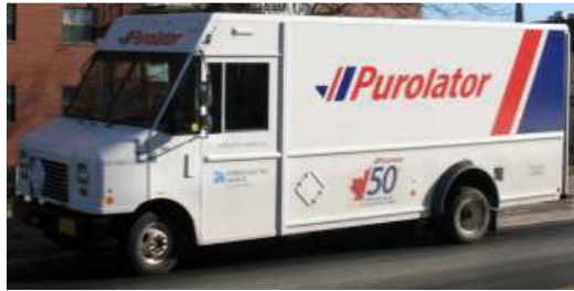
Figure 2 - Azure Dynamics Balance Hybrid Electric Delivery Van (as used by Purolator) Source: Azure Dynamics
