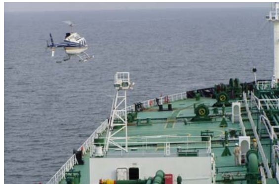
Figure 6.3 Pilot Transfer via Helicopter
