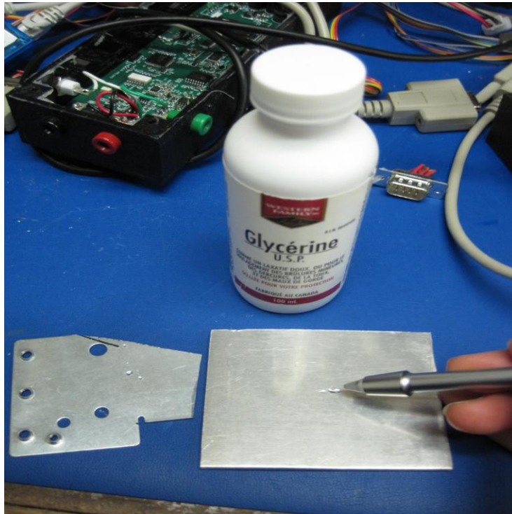
Figure 5-10. Couplant on Target Material
