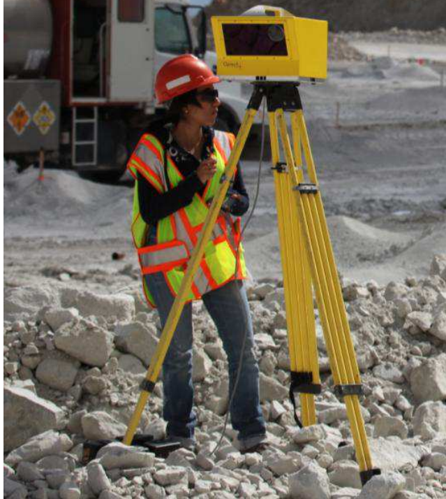
Figure 3 - 6: Optech ILRIS-3D scanner mounted on tripod.
