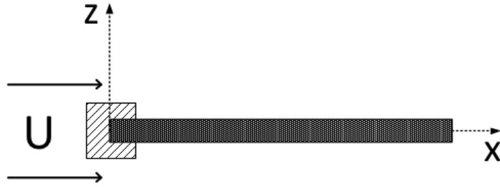
Figure 1: Schematic of a Fluttering Cantilever
