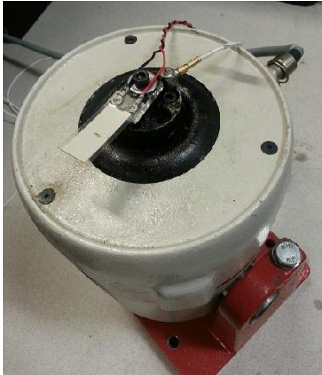
Figure 7: PVDF Mounted on the Shaker Head
