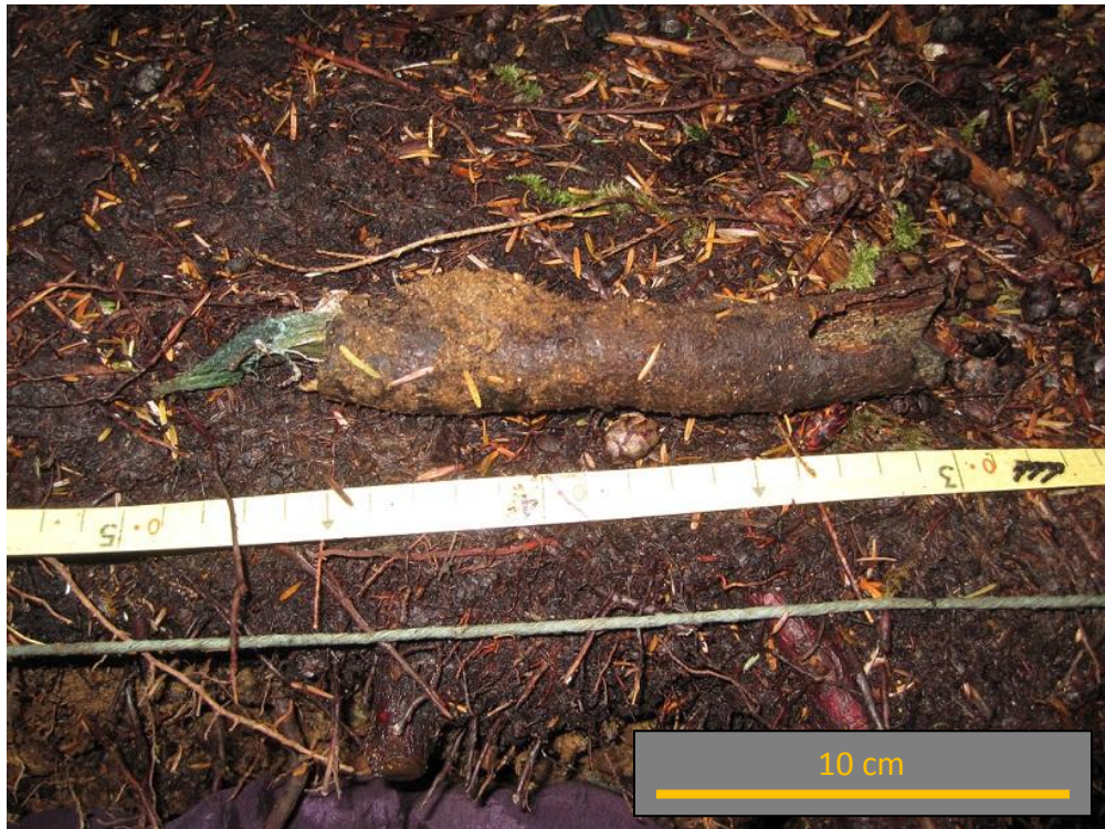
Figure 3.9: Blue dye stains inside a decaying root (SIE 2). Stemflow water flowed laterally through the decaying root.
