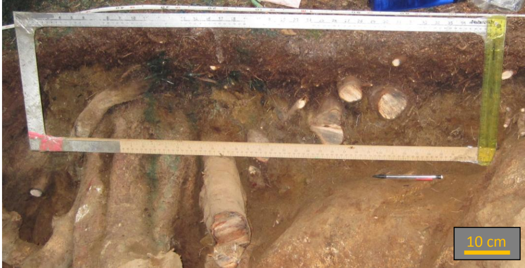
Figure 3.8: Stemflow infiltrated along roots for SIE 2. Dye present in organic surface layer and along roots to depth. Scale of frame is 1 m x 0.3 m.
