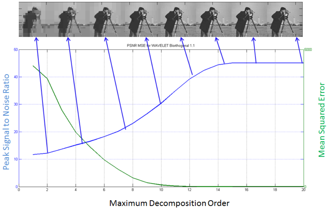
Figure 35 Top)-Psycho-Visual depiction of the reconstructed image using hard-thresholding Bi-orthogonal 1.1 wavelet bases. The arrows show the position of each image on the PSNR (Peak Signal to Noise Ratio) curve for image (Cameraman)
