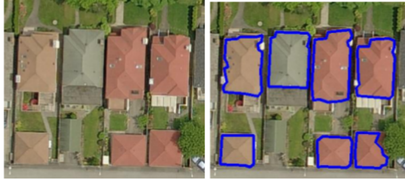
Figure 3.3: Example of the original aerial image, and the extracted rooftop outlines (shown in blue).
