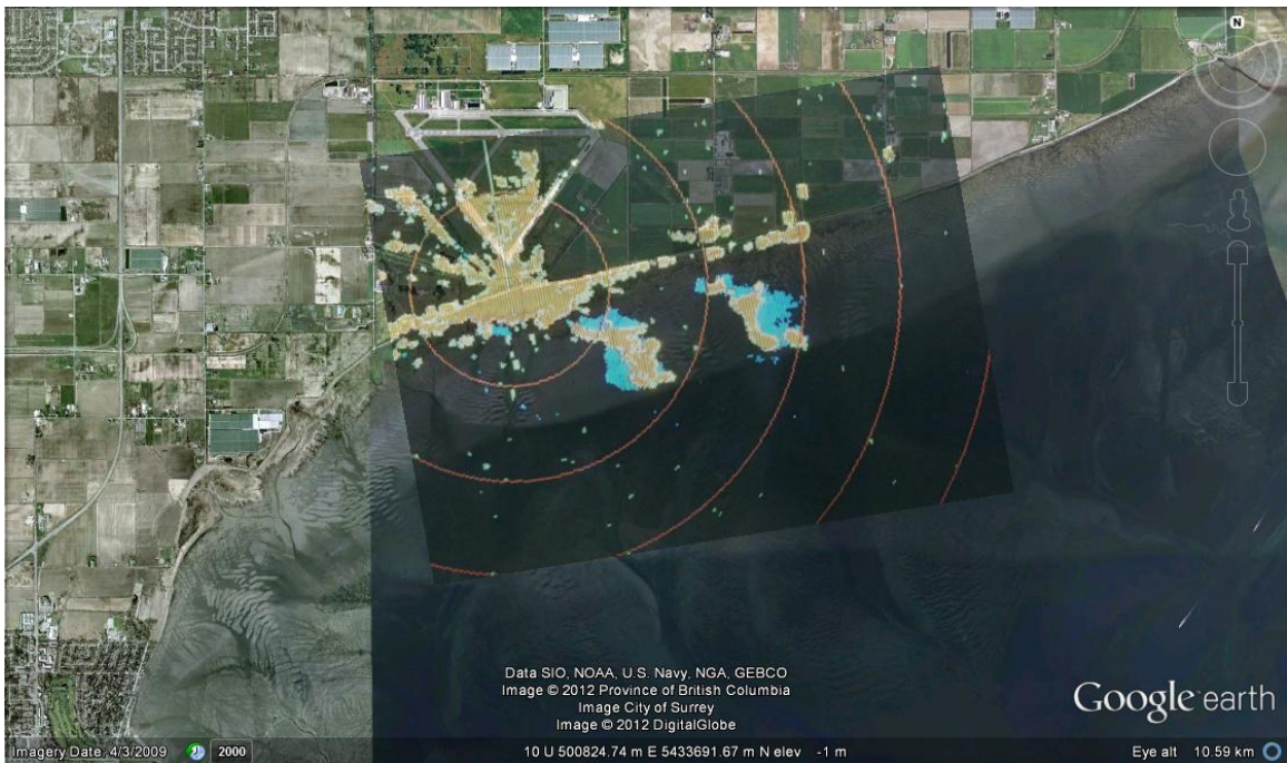
Figure 2-1 Radar screenshot overlaid on Google Earth image of study area. The triangular shape near the centre of the image is the Boundary Bay airport. Large red “blobs” surrounded by blue are the radar visualization of over-ocean flocking dunlins (see Fig. 2-2).
