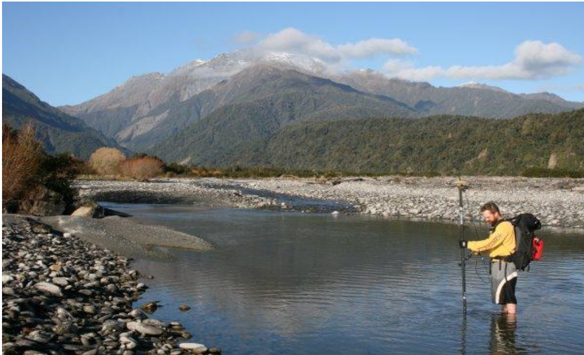
Figure 3.2. Topographic survey of Poerua River just above the SH6 bridge. Data are being gathered by the rover component of the Top Con dGPS system. Mt. Adams is the high peak in the background. (Photograph by Michelle Hanson, 2008).
