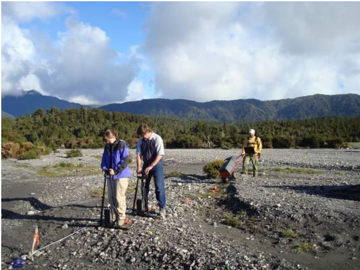
Figure 2.2. Ground-penetrating radar field survey of the Waitangitona River floodplain below the SH6 bridge. In the foreground are two 100 kHz antennae. Data are being recorded in the background on a waist-mounted laptop computer. Photograph by Mauri McSaveney, 2008.
