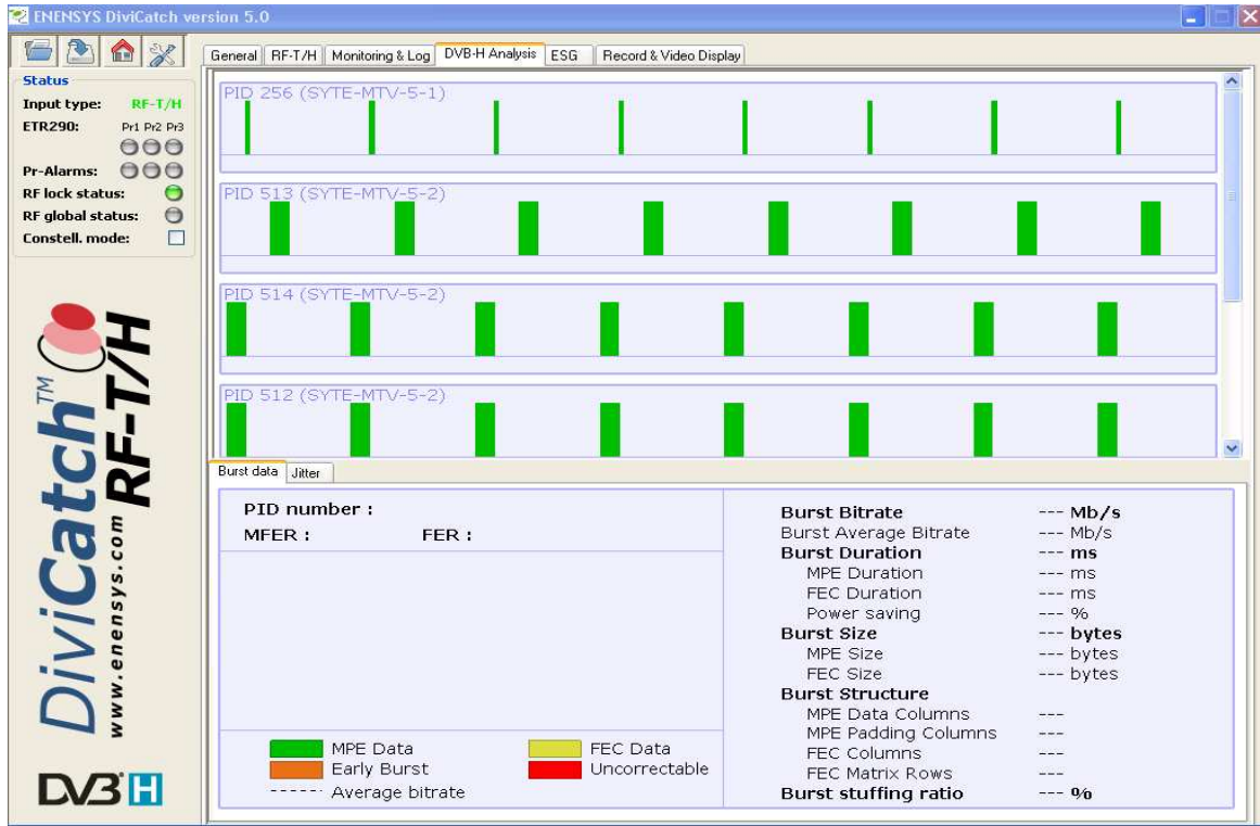
Figure 3.8: DVB-H bursts on Divicatch RF-T/H analyzer
