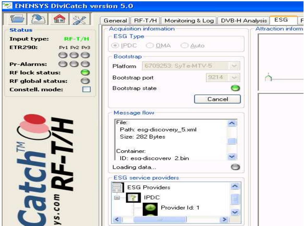
Figure 3.9: ESG information from transport stream on Divicatch RF-T/H analyzer
