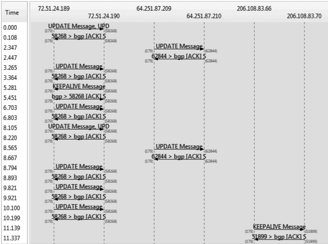
Figure 12. Flow Graph of Collected Traffic. Shown are Time Stamps of Correspondence Between BGP Peer Routers.
