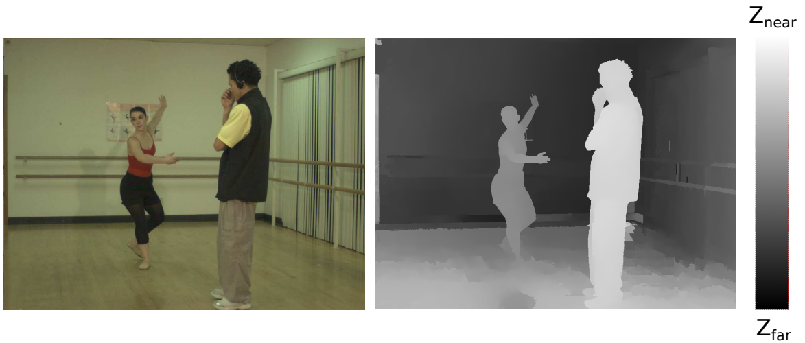
Figure 2.2: This image shows a frame of a 3D video and its corresponding depth map. Depth map is a gray-level image which shows the depth of each pixel
