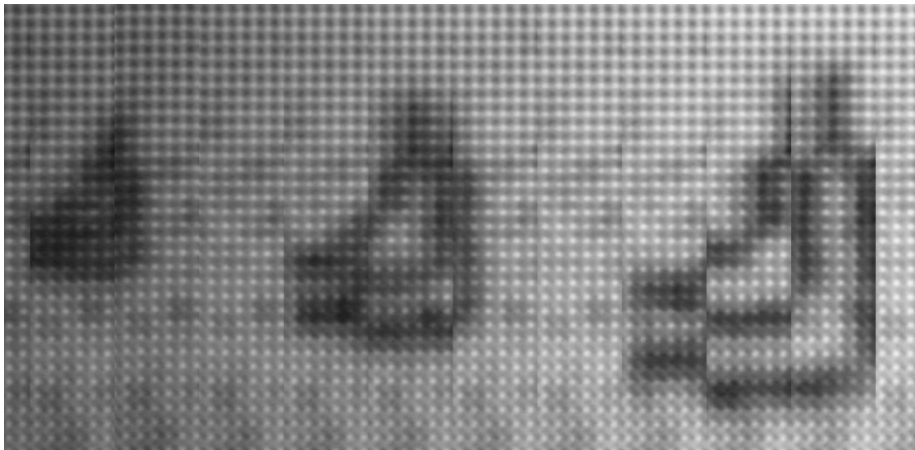
Figure 5-10: ADI with Scattering Medium at SR = 328 ( \text{MTF}_{(200\mu\text{m})}=0.093 , \text{MTF}_{(300\mu\text{m})}=0.26 , \text{MTF}_{(400\mu\text{m})}=0.28 )
