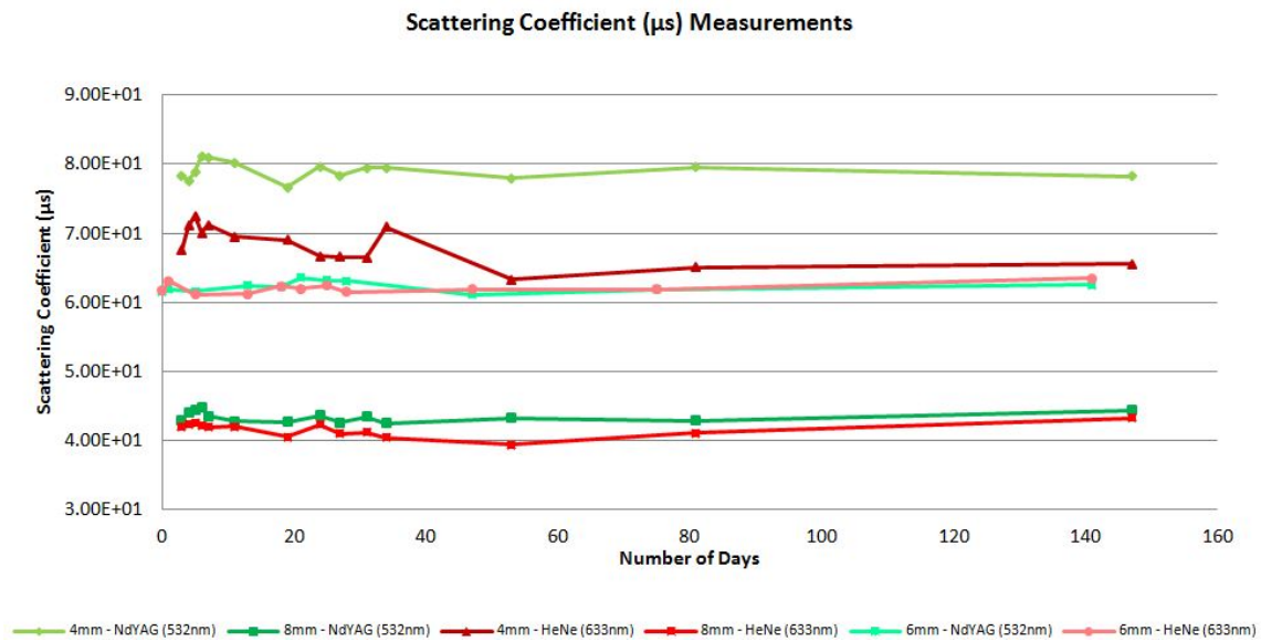
Figure 3-8: Scattering Coefficient measurement with different scattering thickness and wavelength
