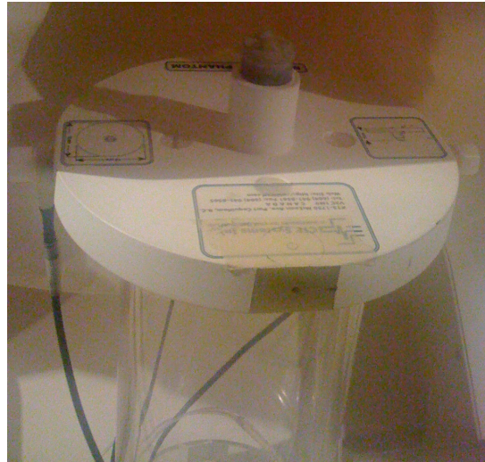
Figure 3.4: CTF Magnetic Dipole Phantom. This phantom consists of a single magnetic dipole located 5cm above the centre of the stand. 4 holes, placed 90 degrees apart along the base of the stand are used to hold head localization coils. These coils form the local "head" coordinate system.
