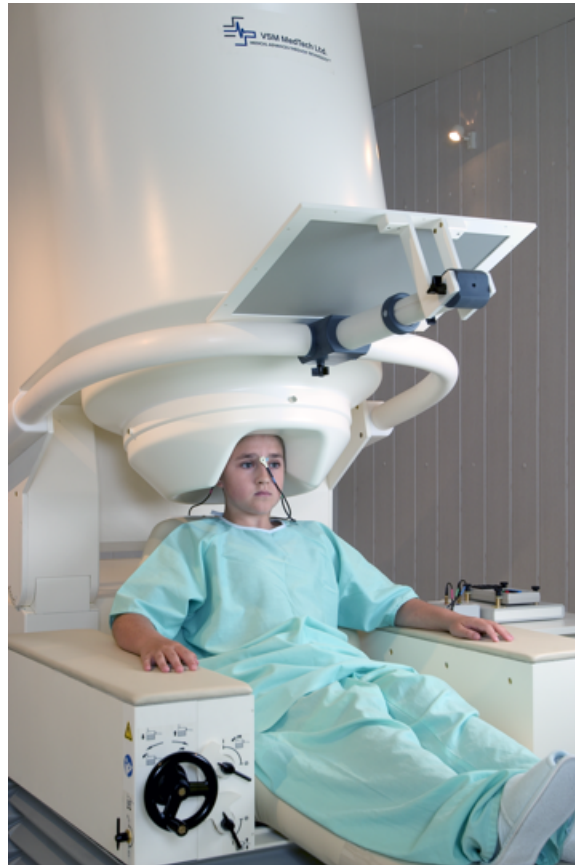
Figure 2.3: The 151 channel CTF MEG System installed at the Down Syndrome Research Foundation, Burnaby, BC.
