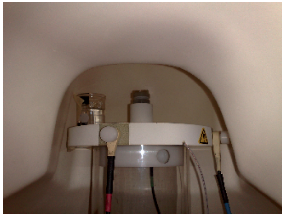
Figure 5.1: Ferrofluid in MEG. The ferrofluid is in the glass beaker water bath (left side of stand).
