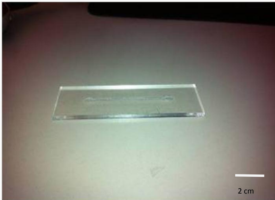
Figure 4-2 Optical Micrograph of Laser Engraved PMMA Micromold
