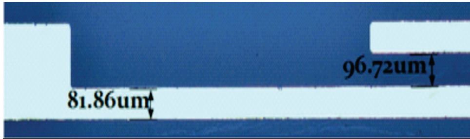
Figure 4-5: One pair of fabricated electrodes
