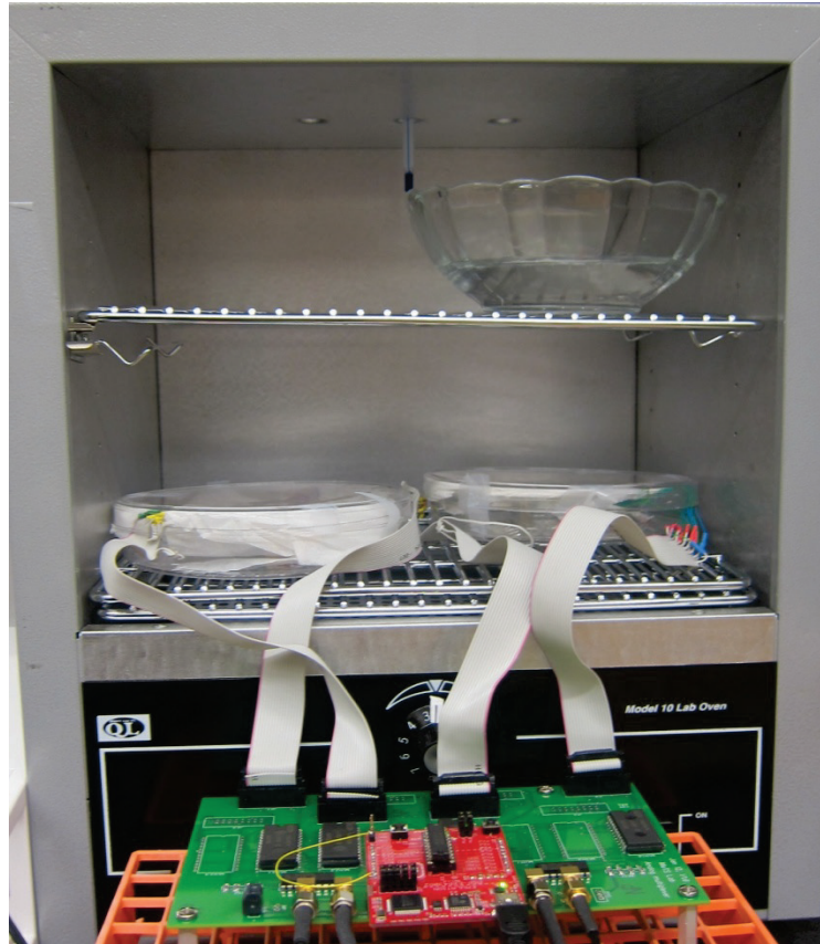
Figure 5-8: Oven used as an incubator to culture bacteria showing a water bowl to maintain humidity
