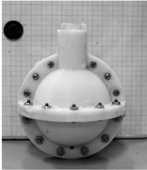
Figure 6-2: The used spherical mould for BSA manufacturing.
