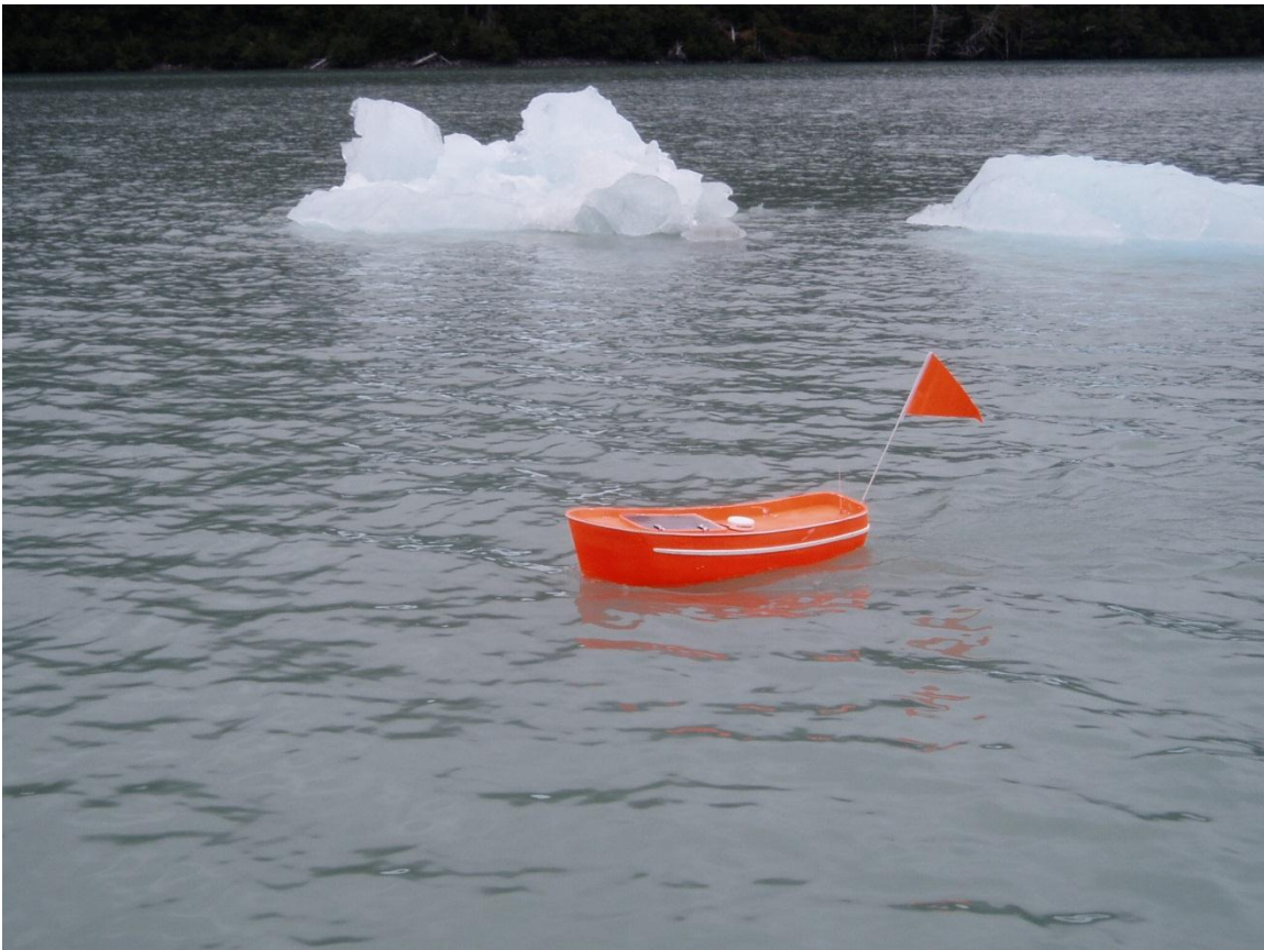
Fig. 5.1. Custom-built, GPS-enabled, remote-controlled boat (85 cm long).
