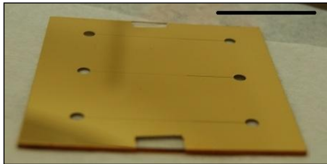
Figure 6: Patterned gold to be used as photo mask during the DUV exposure. The scale bar represents 2.54 cm.
