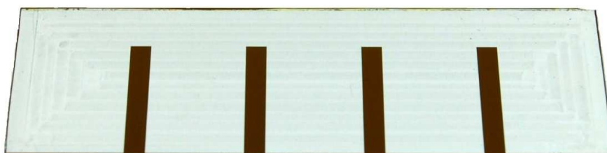
Figure 20: Standard 3"x1" glass slide patterned with the mask shown in Figure 19.
