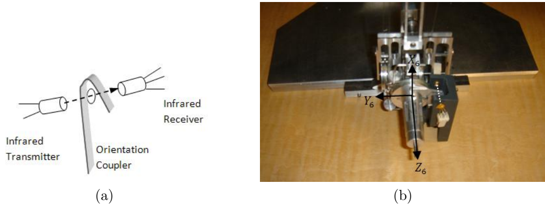
Figure 3.24: Orientation coupling: (a): Orientation coupling by using the mechanical orientation coupler and infrared sensors; (b): A view when the housing of the infrared transmitter and receiver is clamped on the mechanical stand of the end-effector
