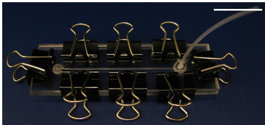
Figure 16: PMMA channel ready for microwave heating with metal clips and input tube attached. Scale bar represents 2.5 cm.
