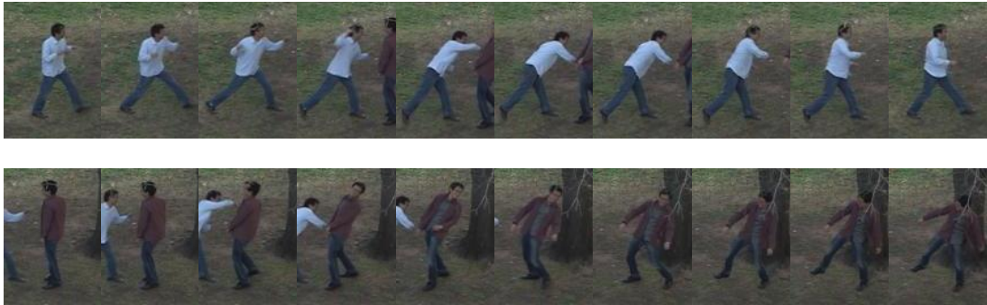
Figure 4.3: Sample trajectories extracted from a 63 frame-long video. The trajectories are the output of our tracker given the human detection in the first frame of the video clip.
