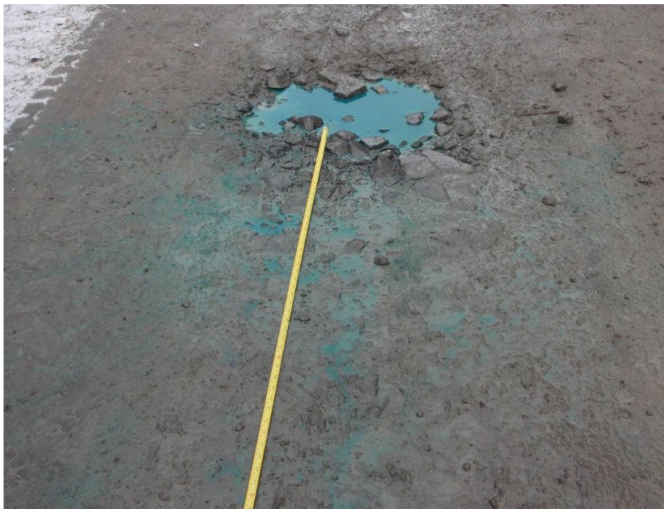
Figure 2.12 Blue dye splashed from a water filled pothole is carried mainly down the road by tires. Lateral splash is mainly within 2.0 m of the pothole
