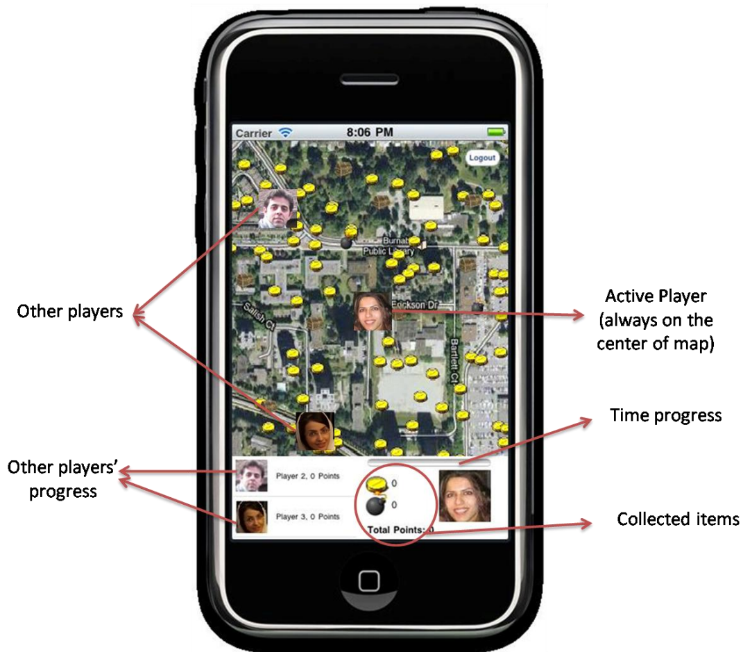
Figure 4.1; A sample screenshot of the Catch Treasures (The rewards are randomly scattered in the environment. To receive each reward, users are required to walk to the location of that reward).
