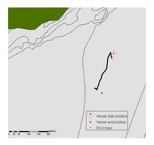
**Figure A2.1:** Example of two data types used for determining track length. The ROV track was interpolated from Trackpoint II data and the vessel positions were recorded in a log at the start and end of the transects. The course corrections at the beginning and end of the ROV track are from the ROV diving and surfacing. The lines are ten meter contour intervals.
