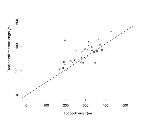
**Figure A2.2:** Relationship between measured track length from the Trackpoint II system and linear distance between vessel positions at the start and end of the transect. The solid line represents the linear regression predicted from the observed data (points).
