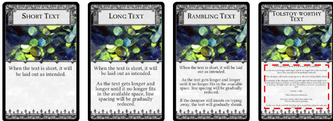
Figure 8.4: Text fitting accommodates unusually long rules with ease. As the text gets longer (from left to right), the layout engine will first reduce line spacing and then scale the text size down. When the scale factor becomes extreme, a red warning box is displayed.
