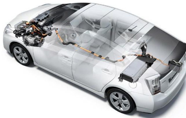
Figure 3-5. Power Source Connection of a Toyota Hybrid System [74]
