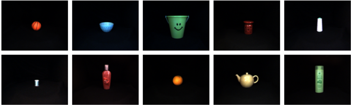
Figure 5.4: Objects Generating False-Positive Matches. The 10 objects with the most false positive matches within the cross-database testing are shown. The common trait among these objects is that they are composed of only one dominant color. This demonstrates an important limitation in the object recognition algorithm.
