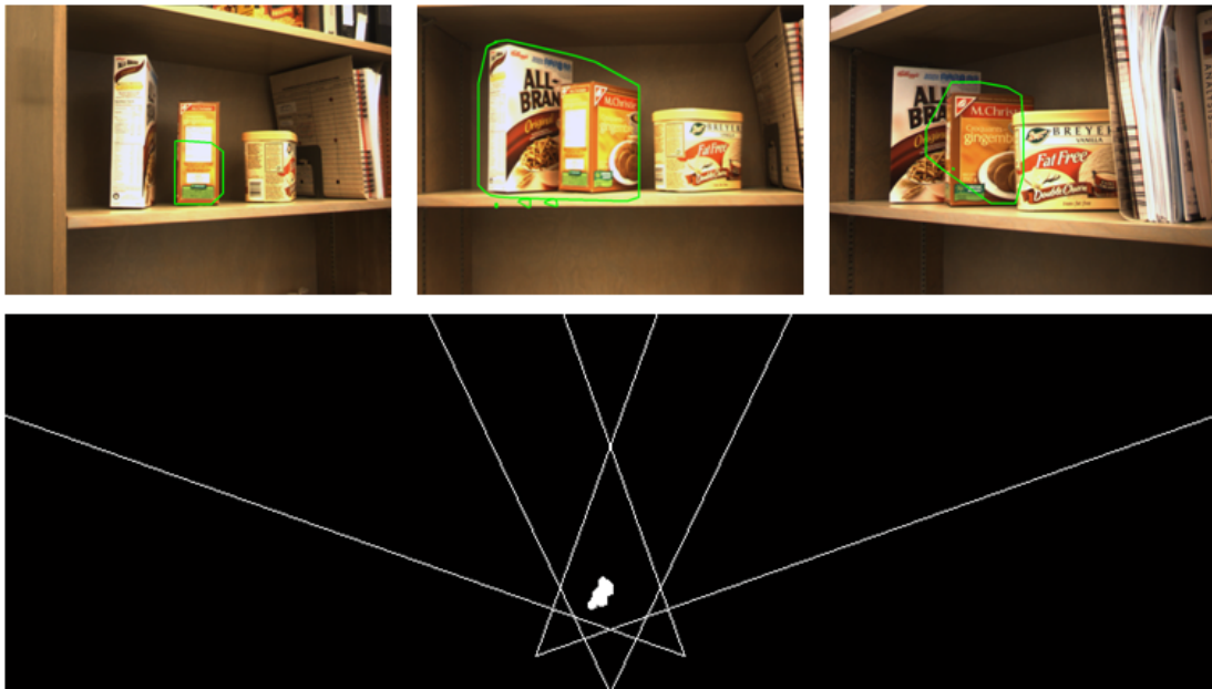
Figure 5.16: Multi-View Inspection Results - Gingersnaps. The matching results are shown along with the resultant birds-eye view confidence map.
