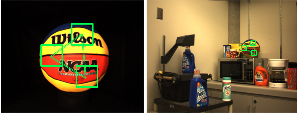
Figure 4.17: Triangular Constraint Example. Three image patches extracted from the scene image (right) are matched to the model image (left). The distances between the image patches in the scene are consistent with the image patches in the model, thus passing the triangular constraint.
