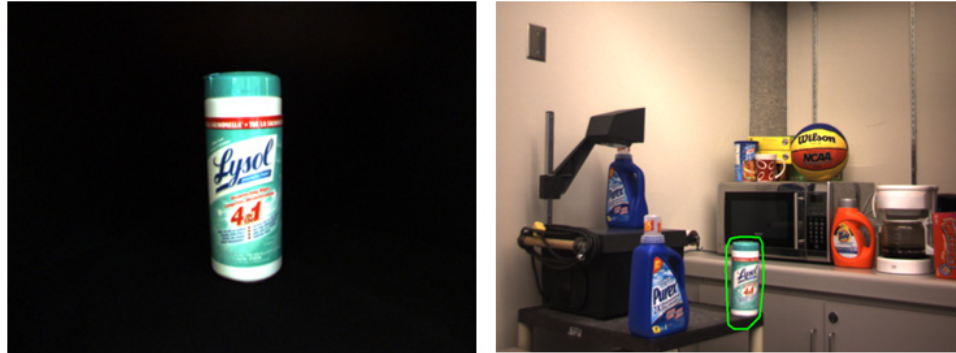
Figure 1.1: Recognizing and Locating an Object. Appearance information extracted from the model image of the object ( left ) is used to recognize and locate an instance of the object in a scene image ( right ). The located region is outlined in green.
