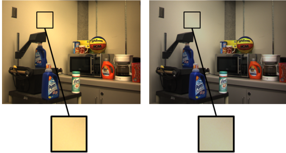
Figure 4.12: Illumination Compensation. Left : Original scene image with a sample patch isolated for demonstration. Right : Scene image after applying the illumination compensation stage again with sample patch isolated. The difference in color is clearly seen when comparing the isolated patches.
