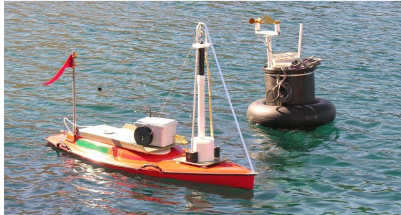
Figure 5.1: Application: the USC/UCLA NAMOS robot boat: a mobile aquatic observatory with anchored buoy base-station. A docking/recharging system is under development.
