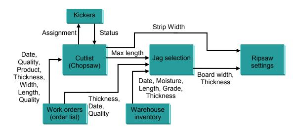
Figure 2.3 Flow of information in the rough mill
