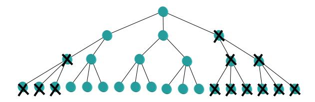
Figure 6.4 If one node is infeasible solution, the rest of the sub-tree nodes are infeasible solutions too
