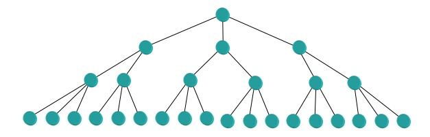
Figure 6.3 Search tree for three variables: variable1 has three domain values, variable2 has two domain values and variable3 has three domain values
