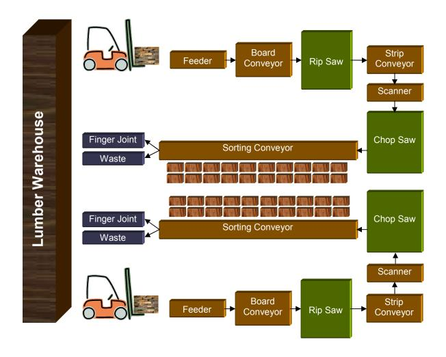
Figure 2.1 Rough mill production lines: Forklifts transfer jags from the warehouse to both ripsaws. Chopsaws cut wood into components of specific sizes.
