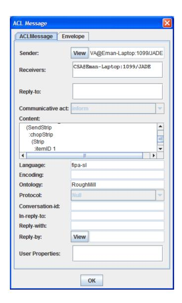
Figure 5.6 ACL message containing a strip sent from the conveyor agent to the chopsaw agent
