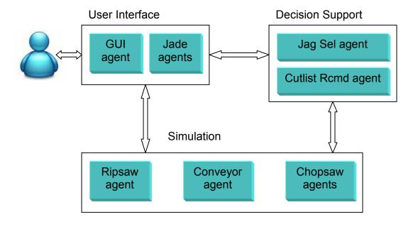
Figure 5.3 System architecture showing different types of agents
