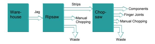
Figure 2.2 Flow of lumber in the rough mill
