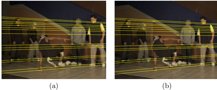
Figure 2.2: A pair of images with superimposed correspondences and their epipolar lines. (a) Left view; (b) Right view.
