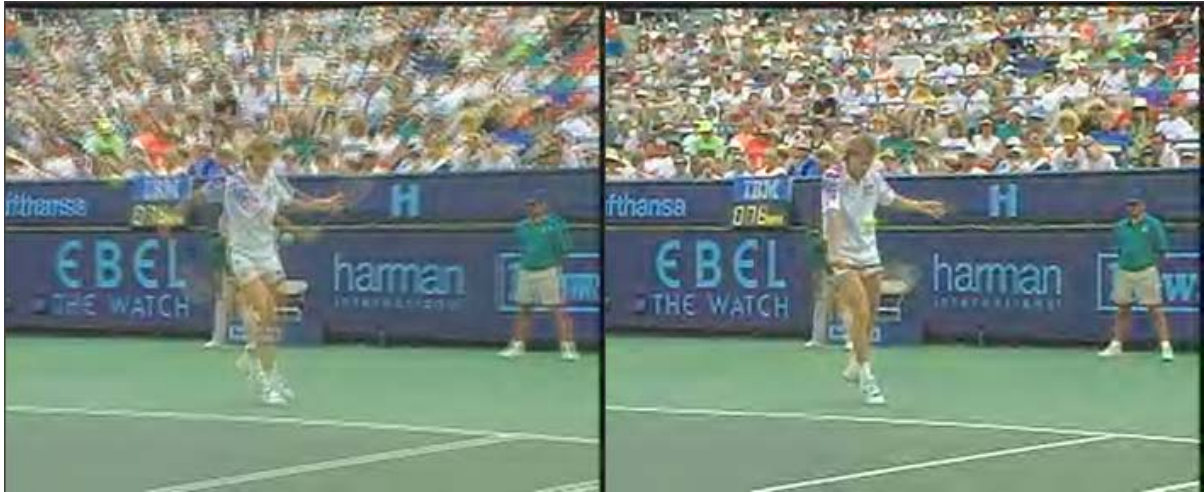
Figure 3.6: Frame reconstructed by zero-motion error concealment (left) and the coded loss-free frame (right)
