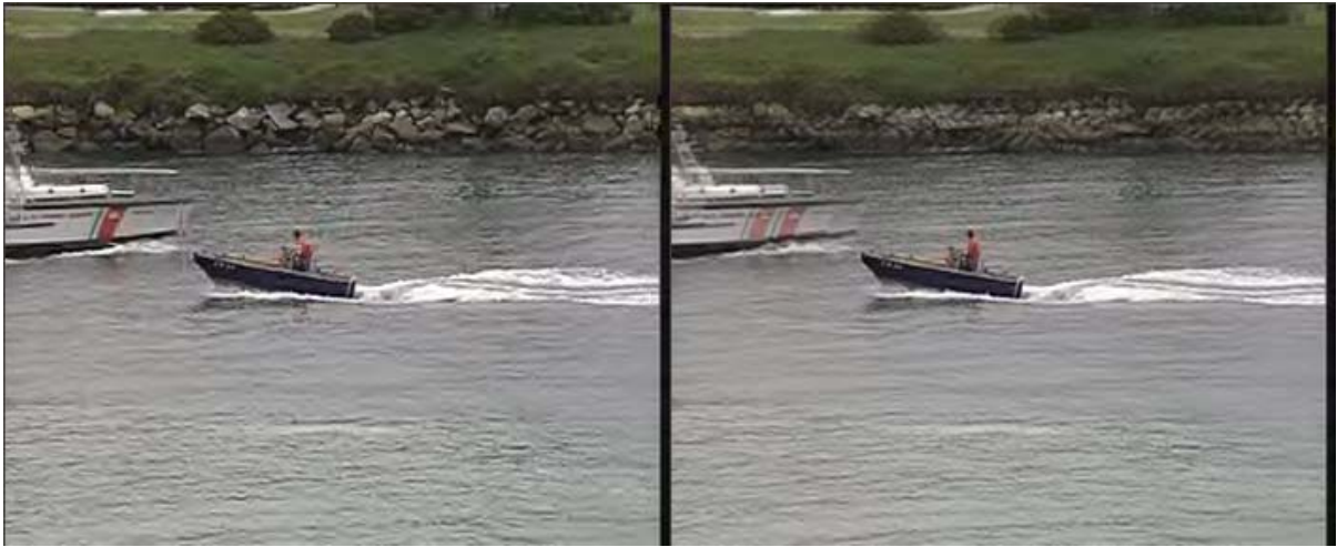
Figure 4.4: Frame that is reconstructed by complete error concealment (left) and by zero-motion error concealment (right) in one-level MCTF
