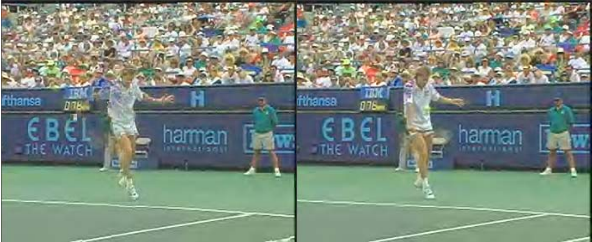
Figure 3.7: Frame that is reconstructed by motion concatenation followed by motion re-estimation and zero-motion error concealment (left) and the coded loss-free frame (right)
