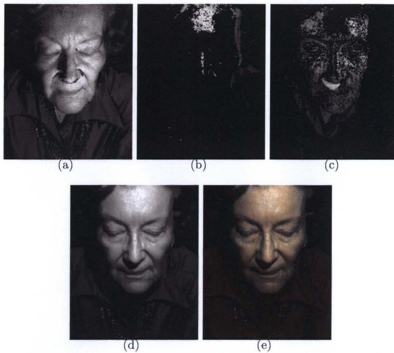
Figure 6.4: Chromaticity-based method. (a): Approximated matte contribution. (b): Modeled sheen contribution. (c): Modeled shade contribution. (d): Reconstructed luminance image of the input data. (e): Reconstructed colored image of the input data.
