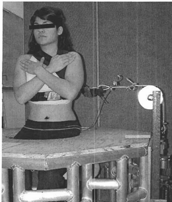
Figure 3.2 Subject in apparatus pulling in lateral flexion
