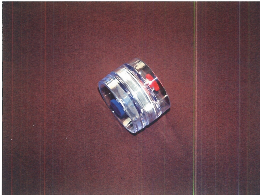
Figure 3. Passive monitor as sealed for transport and storage
