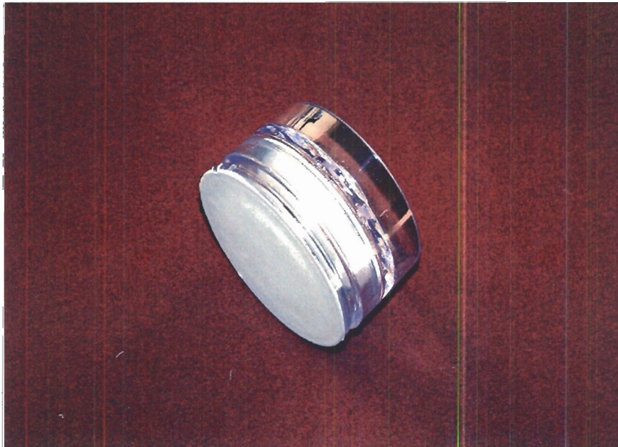
Figure 2. Passive monitors for nicotine sampling as constructed.
