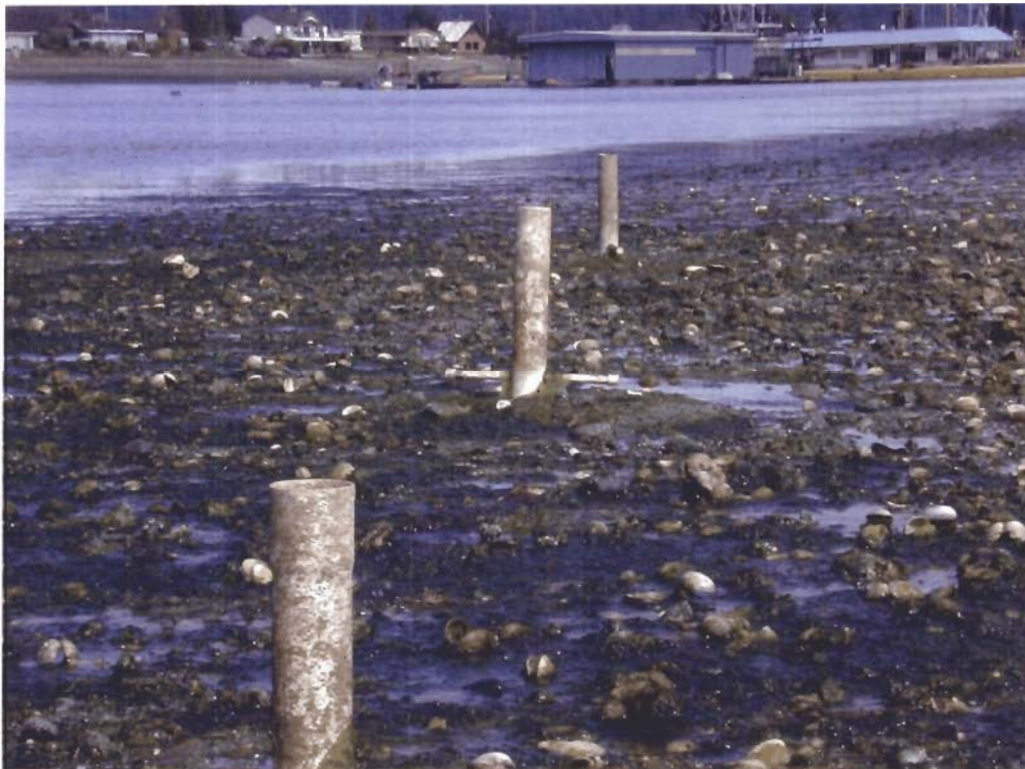
Figure 4.3: Sediment traps deployed at Deep Bay.
