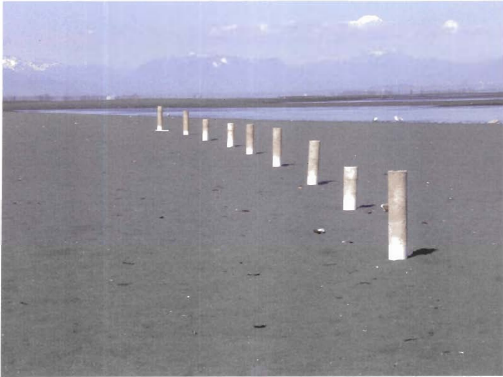
Figure 4.2: Sediment traps deployed at Boundary Bay.
