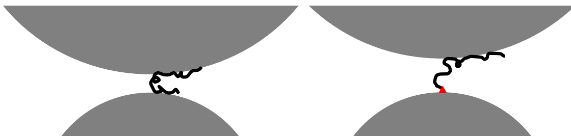
Figure 4.4: Left: diagram of an elastin molecule tethered non-specifically between two beads. Right: diagram of elastin molecule specifically linked to one bead and non-specifically bound to another.
