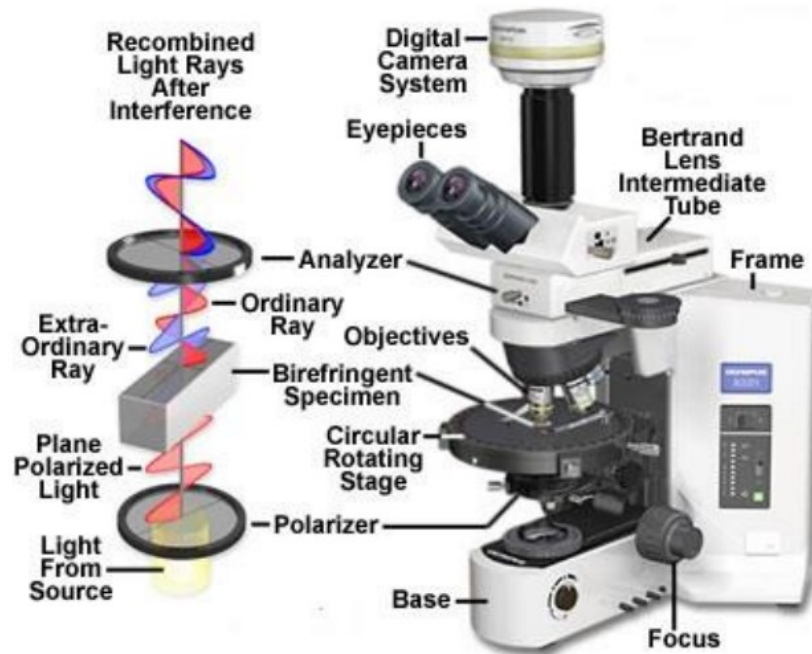
Figure 2.8: Principle and configuration of polarized light microscopy (PLM).
