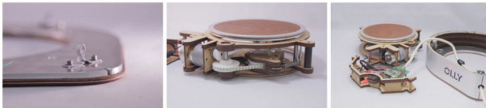
Fig. 6 From left to right. The exterior enclosure included a cabinet bracket for easy access to internal components during maintenance visits; the belt that actuates Olly's rotational movement using a stepper motor; Exploded view of various modular components that fit within Olly's alumni enclosure when assembled
