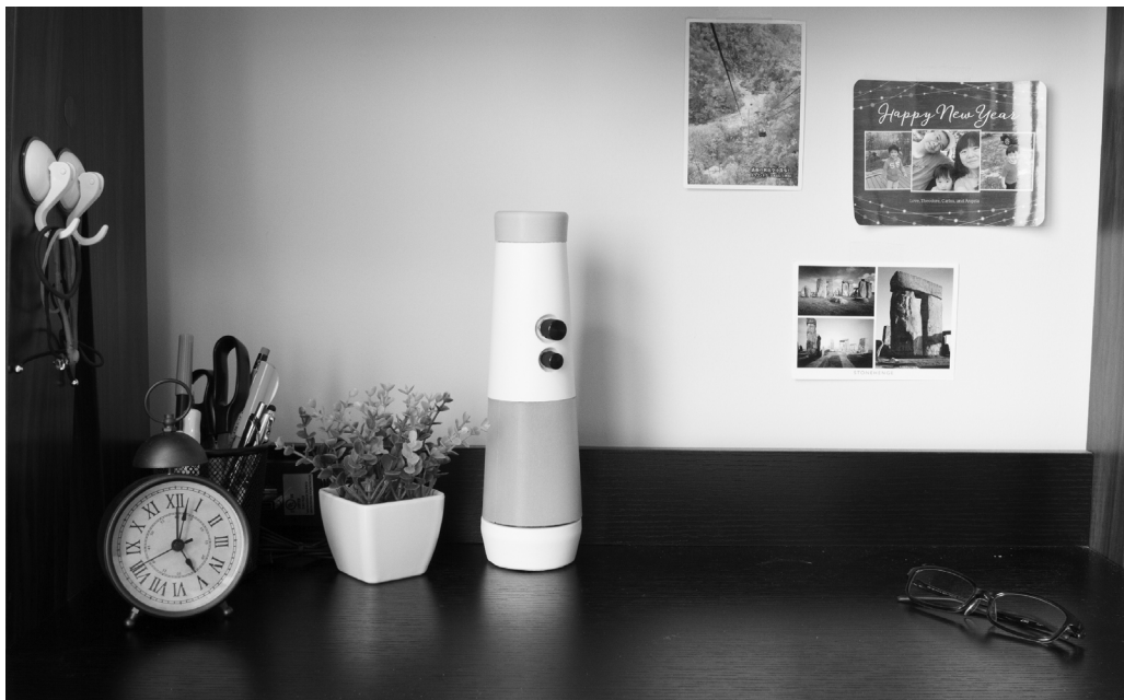
Figure 1 Leveraging the metadata of each digital photo, Chronoscope is a tangible device that enables interactions through and across time in one’s personal photo archive. The scope form and the monocular feature are designed to suggest its user a consciously focused viewing experience.
