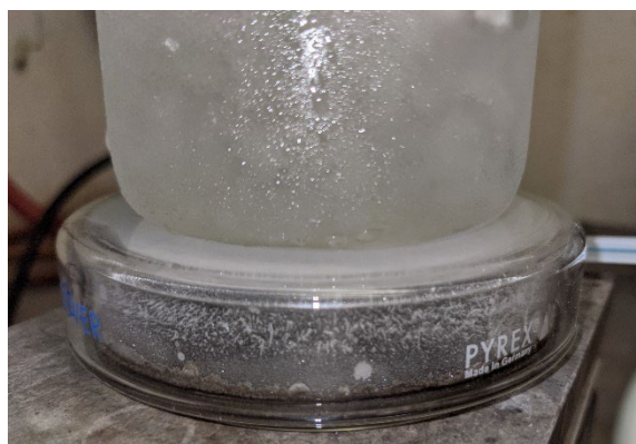
Figure S3: Side view of the sublimation process (Ice filled beaker on top of a Petri dish cover, which is on the Petri dish bottom). Notice the crystallization occurring on the side of the Petri dish bottom. These crystals need to be scrapped back into the middle of the dish.
