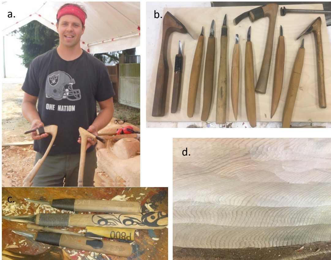
Figure 2.4. Pictures of (a) Karver Everson holding traditional adzes, and (b) and (c) other traditional hand tools made and used by carvers in their practices today. The use of such tools is the most efficient and effective on old growth LCC with tight grains, shown in (d) (photo credits: Julie Nielsen).
