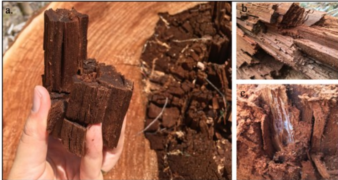
Figure 3.6. Pictures of redcedar heartwood that has been decayed by white rot and brown rot fungal species (photo credits: Kryz Stone). Pictures (a) and (b) show heartwood characteristic of decay caused by brown rot fungi. Picture (c) shows heartwood characteristic of decay caused by white rot fungi.
