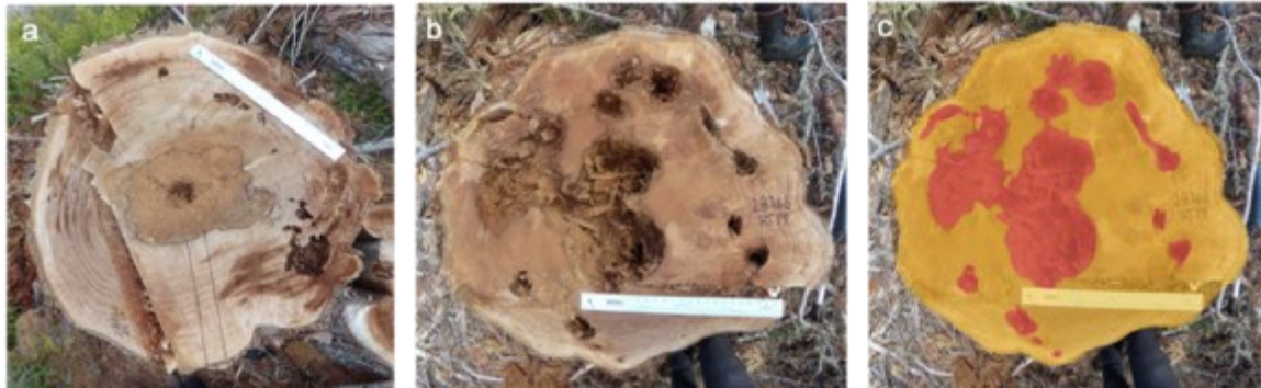
Figure 4.5. Plan-view pictures of two LCC stump surfaces showing (a) an area of incipient decay delineated in marker and (b) areas of advanced decay with missing wood (photo credits: Krys Stone). Picture (c) illustrates the use of the program Affinity Photo to obtain a ratio of (pixels of) decayed wood, highlighted red, to (pixels of) sound wood, highlighted yellow, for the stump pictured in (b) (photo credit: Krys Stone).
