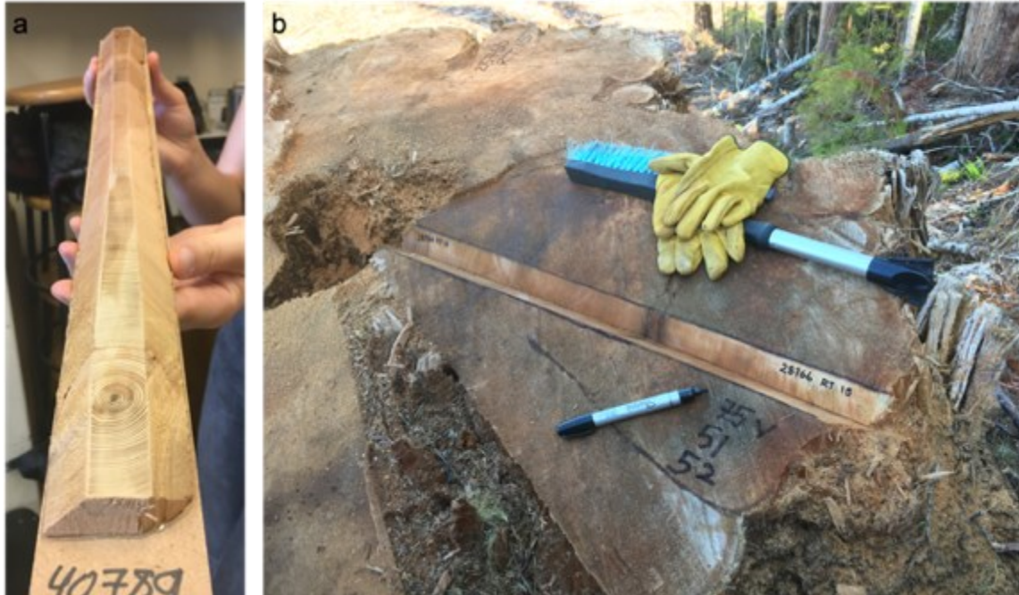
Figure 4.6. Pictures of (a) a cross-sectional sample of wood cut from the radius of a LCC stump after sanding and, (b) a radial section of a LCC stump where a sample was removed (photo credits: Kryss Stone).
