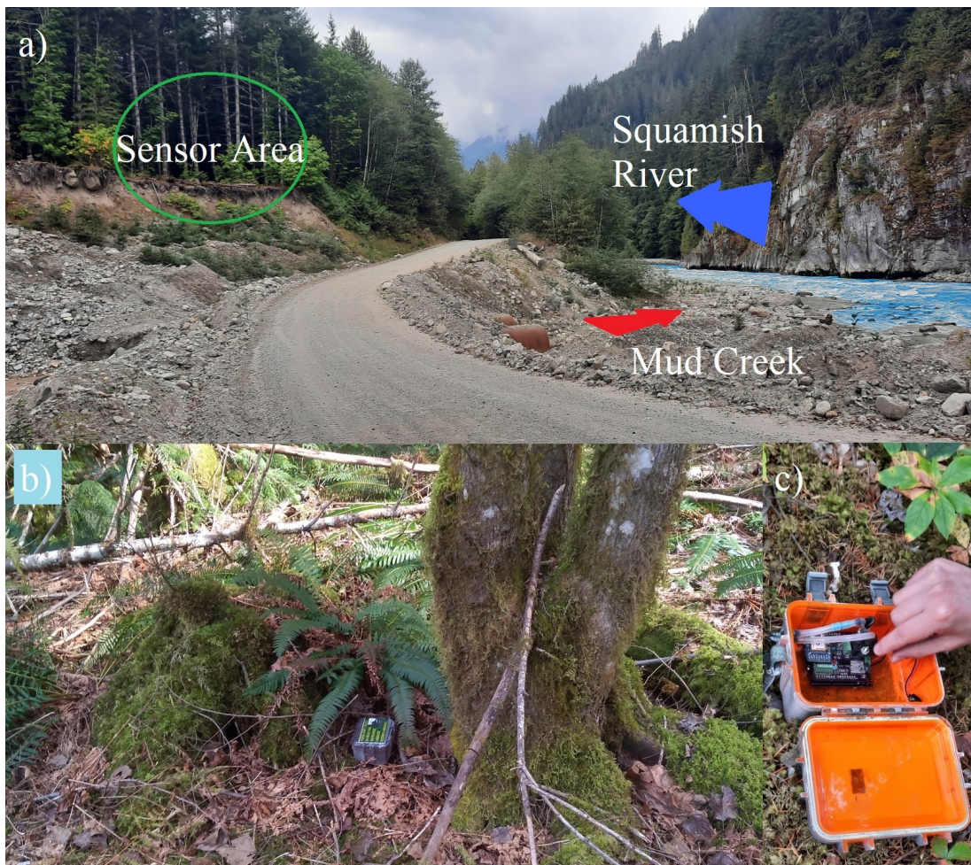
Figure 4.3: Collage of images showing the installation setting of the Gem acoustic sensor. See Figure 4.2 for site location.
