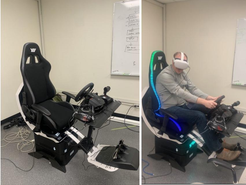
**Figure 15. Yaw2 simulation chair with Logitech G-Series wheel and pedals attached (left) and Dr. Nick Hedley using DRIVR.**
