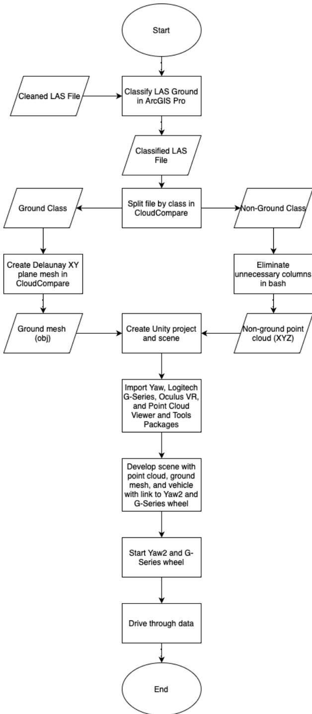
**Figure 12. Workflow for the development of an immersive data experience including collected point cloud data, the Yaw2 simulator, Logitech G-Series wheel and pedals, and Oculus Quest 2.**
