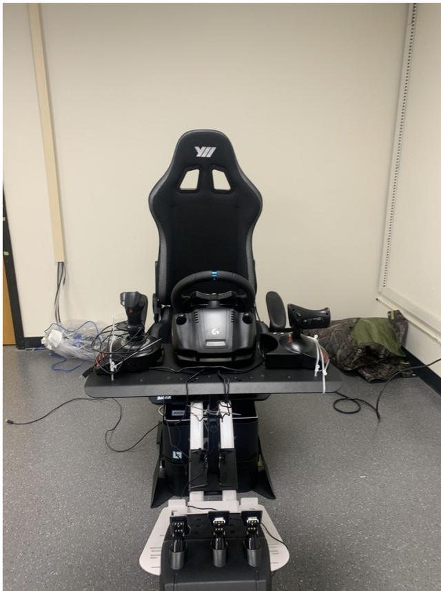
**Figure 13.** The Logitech G-Series wheel and pedals are connected to the Yaw2, which is in turn connected via USB to the laptop to the left of the image.
