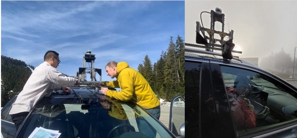
**Figure 3. 3DMS: a vehicle-mounted mobile data acquisition system, combining LiDAR, Stereo camera imaging and GPS.**
