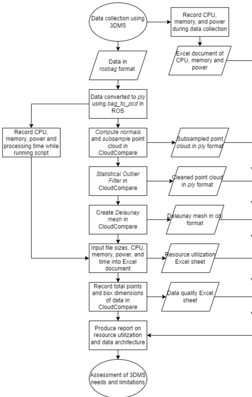
**Figure 5. Workflow diagram of the assessment of resource utilization and data architecture used as the overarching methodology.**
