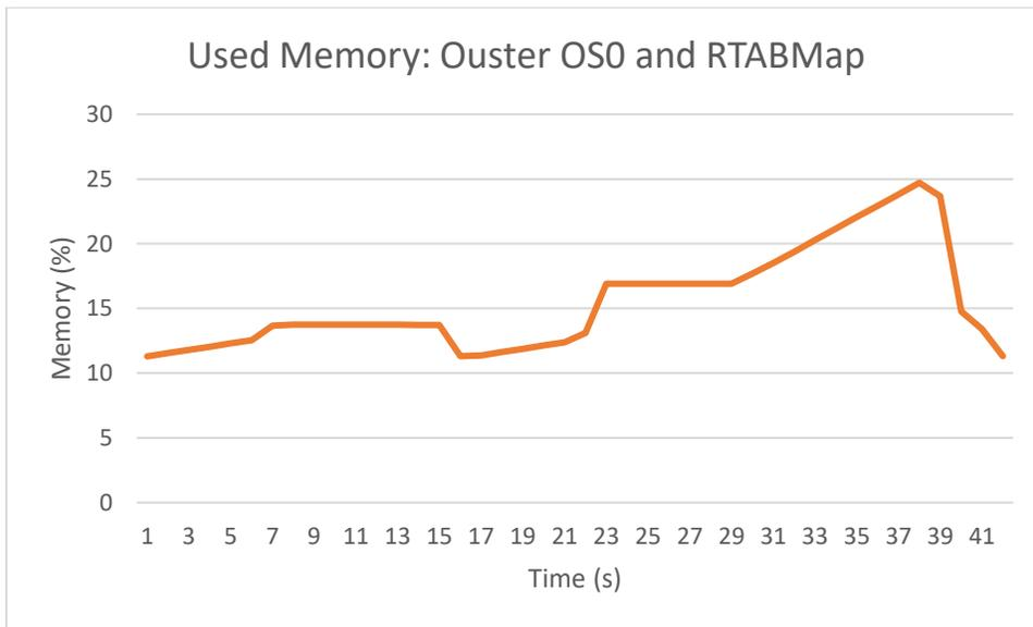
**Figure 7. Used memory while running the Ouster OS0 and RTABMap simultaneously.**
