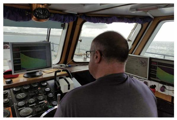
Figure 3 Interior of the hydrographic small boat carrying out multibeam surveying (Institudo Hidrografico).
