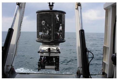
Figure 4 ROV Launch and Recovery System with winch and A-Frame. (Brazilian Navy).
