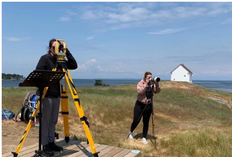
Figure 6. Primary observers using the theodolite and mirrorless camera to track a whale event detected in the LBCO survey on June 3, 2023. Photo credit: Lauren Laturnus.
